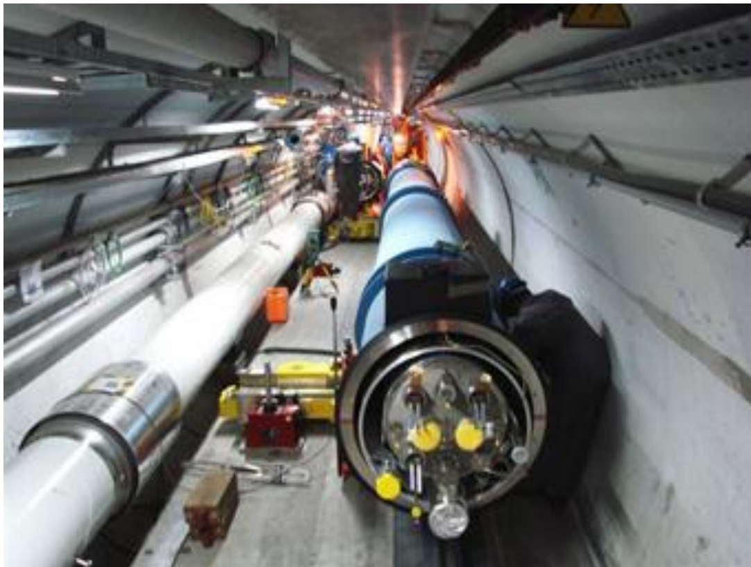
Superconducting magnet section number 1000 for LHC was installed on 5 September 2006 in the 27 km long underground tunnel close to Geneva.
