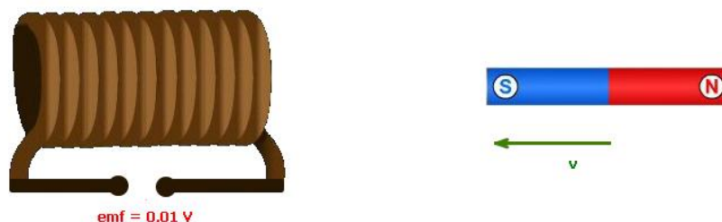
Figure 20. Induced EMF from moving magnet
