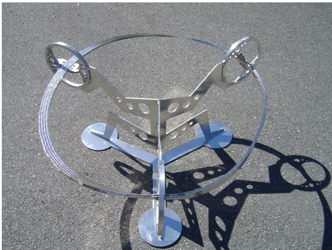
Möbius-shaped magnetic track for levitating train. Photo credits: Vegard Farstad
